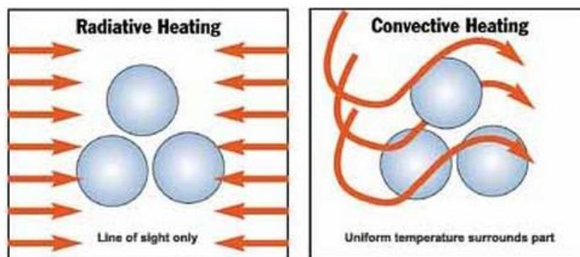
*Figure 4. Radiative heating process and convective heating process*
