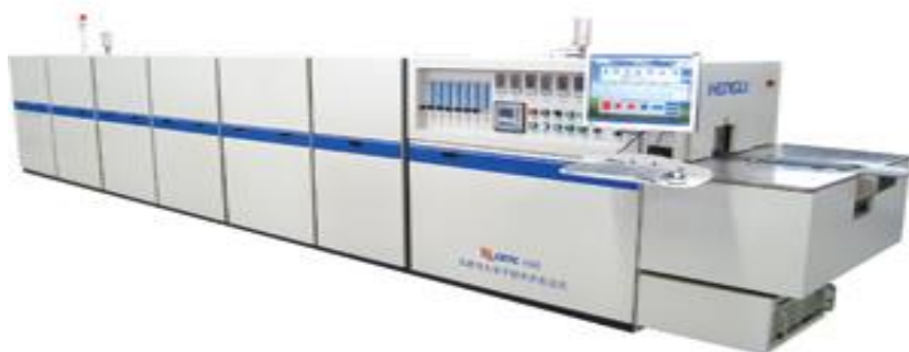
Figure 4: Hengli HSA series belt furnace
