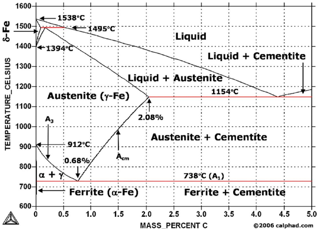
Fig 2. Fe-C phase diagram (Courtesy of online source <http://www.calphad.com/iron-carbon.html>)
